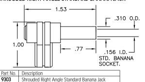
Fits most **TRIPLETT** Instruments with recessed plugs for shrouded receptacles. **Construction:** Nickel-Plated Beryllium Copper Spring Socket. Plastic Handle. Solderless Assembly. Colors: Red, Black.
