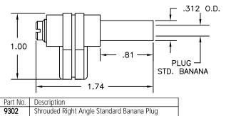
Fits most **FLUKE** and **B&K PRECISION** Instruments with recessed receptacles for shrouded plugs.
