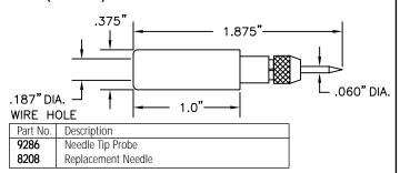
**Construction:** Plastic Handle. 1/4-32 Threaded Assembly. Solder Connection. Nickel Plated Brass Collett. Phono Needle Point. Colors: Red, Black.
