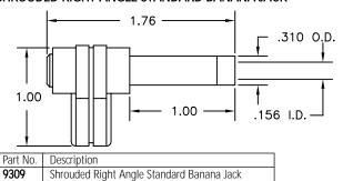
Fits most SIMPSON Instruments with recessed plugs for shrouded receptacles.
