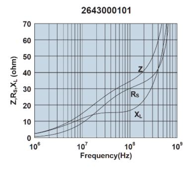
Impedance, reactance, and resistance vs. frequency.
