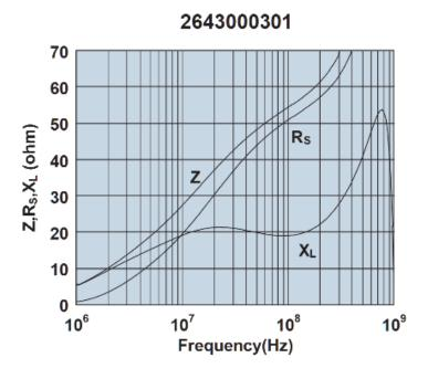
Impedance, reactance, and resistance vs. frequency.
