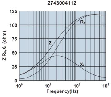
Impedance, reactance, and resistance vs. frequency.
