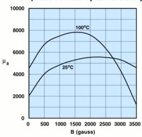
Measured on an 18/10/6mm toroid at 10kHz.
