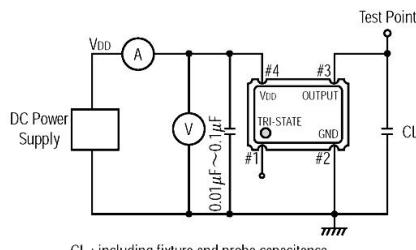
CL : including fixture and probe capacitance.
