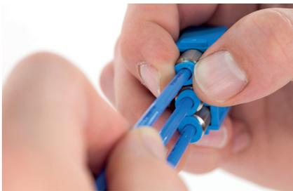
3. In order to remove the pneumatic hose from a pneumatic contact that uses Push-In termination, press the contact's blue ring while pulling on the hose.
