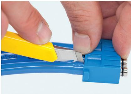
4. In order to remove the pneumatic hose from a pneumatic contact that uses the ID termination technique, cut the hose along its gripping surface. The hose can then be removed from the pneumatic contact.
