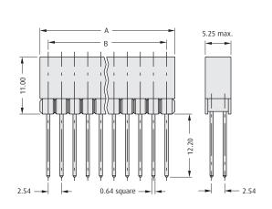
Press-Fit connector M20-615 supplied with spacer moulding M20-614
