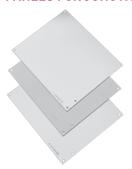
Steel panels are 14 gauge, finished with white polyester powder paint or with a conductive, corrosion-resistant coating. Stainless steel panels are 14 gauge Type 304 and have a commercial #2B finish which is protected on one side with a plastic film. Aluminum panels are 5052-H32 aluminum alloy 0.080-in. (2-mm) thick and protected on one side with a plastic film. Panel mounting hardware is furnished with all enclosures which accept these panels.
