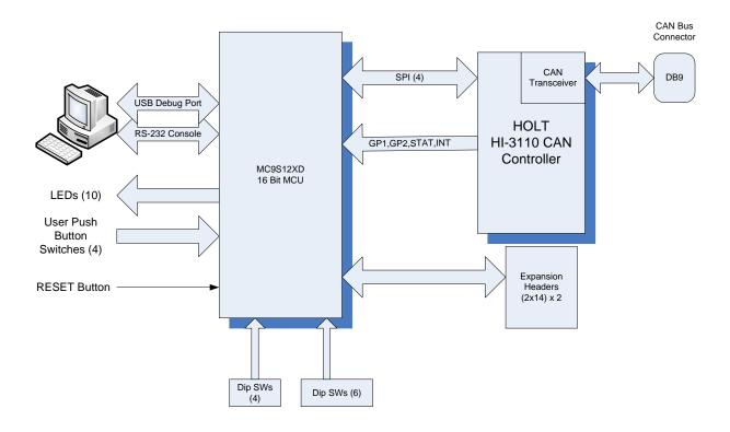
The board requires a +5V (0.5A) power supply applied to TP1 and Gnd to TP6. There are two ways to connect the CANL and CANH signals to the CAN Bus. The CANL and CANH Bus signals are available on the two test points on the top right side of the board or from the DB9 connector.
