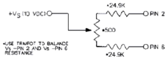
Figure 2 Sensing Bridge Supply Circuit
