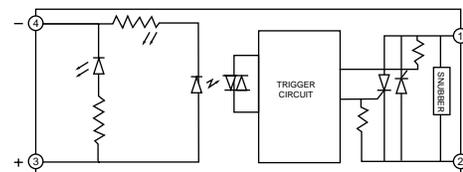
DC INPUT EQUIVALENT CIRCUIT
