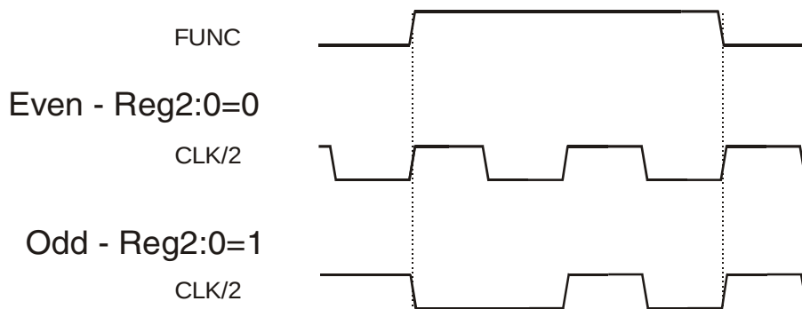
Figure 12-5 CLK/2: Even versus Odd
