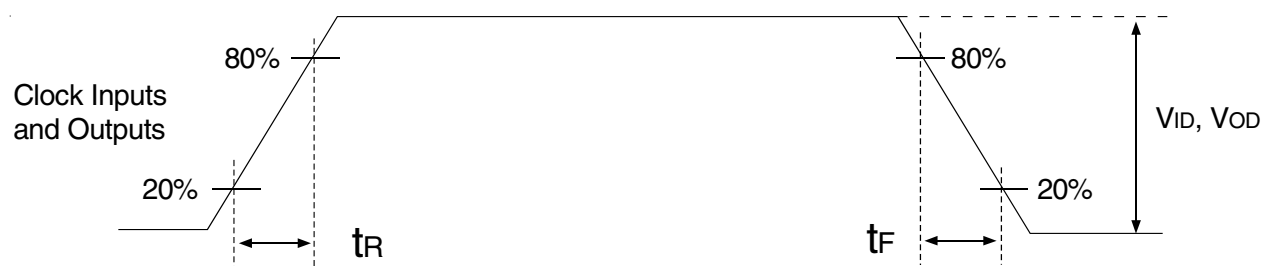
Figure 8. Input and Output Slew Rates
