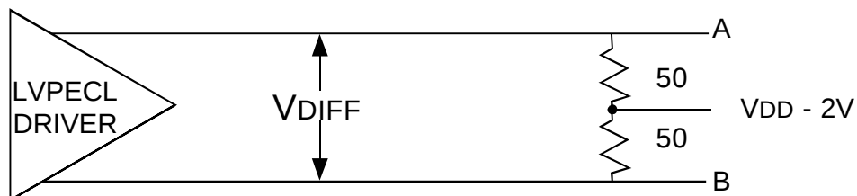
Test Circuit for LVPECL Output Characteristics
