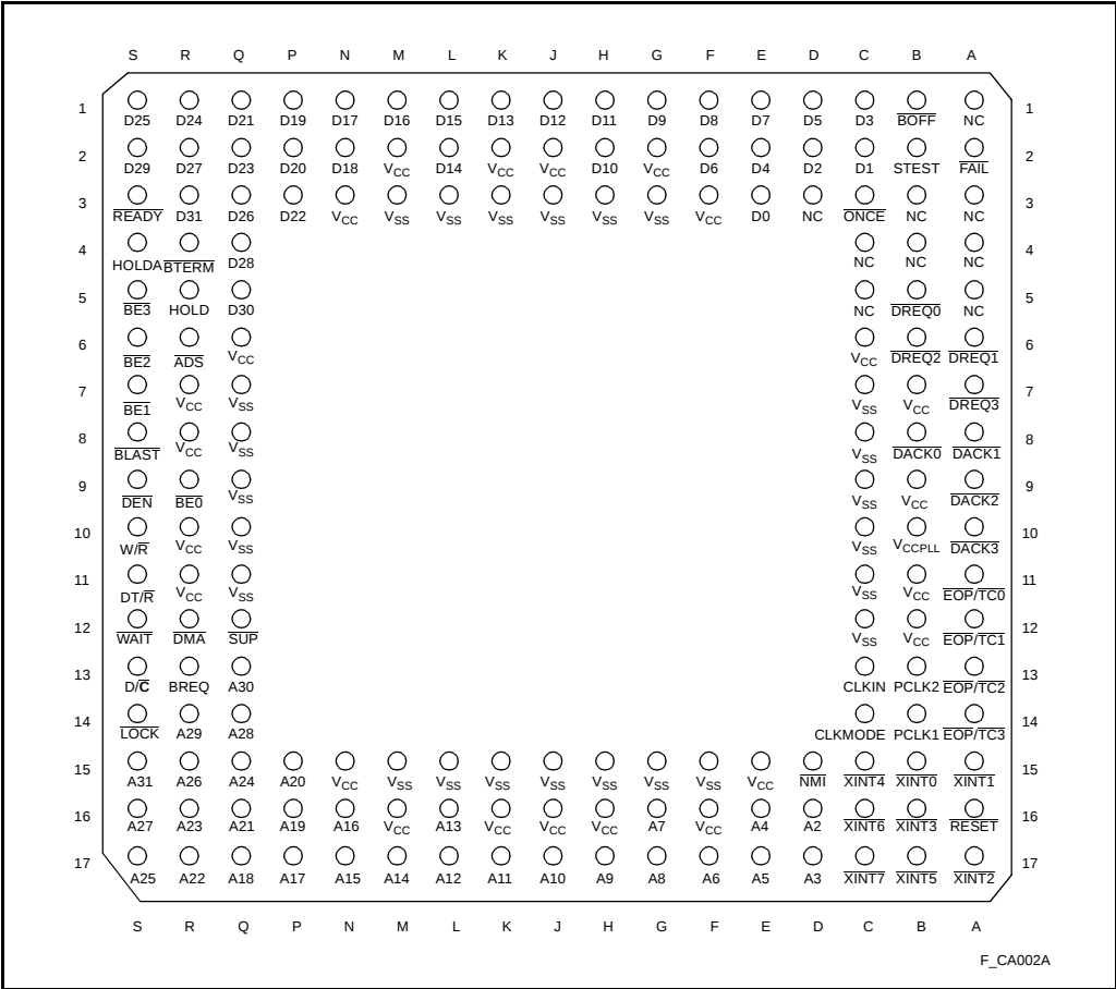
Figure 2. 80960CF PGA Pinout—View from Top (Pins Facing Down)
