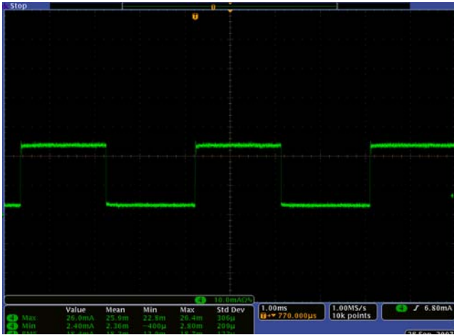
FIGURE 12. I LED AT 50% PWM DIMMING
