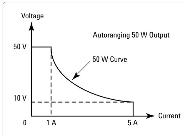
Therefore, this 50 W autoranging power supply, due to its extended voltage and current range, can produce voltage and current combinations in the range of a 250 W non-autoranging power supply.
