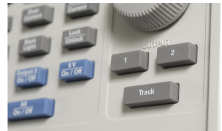
Figure 3. Simplifies Output 1 and Output 2 setup with tracking feature
