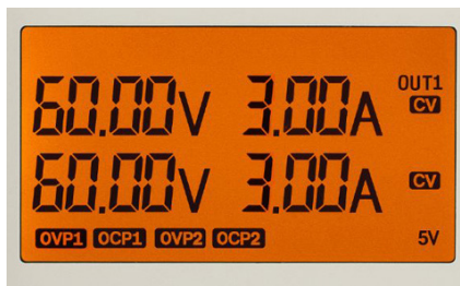
Figure 2. Backlight on/off feature with dual reading (voltage and current) on an LCD display
