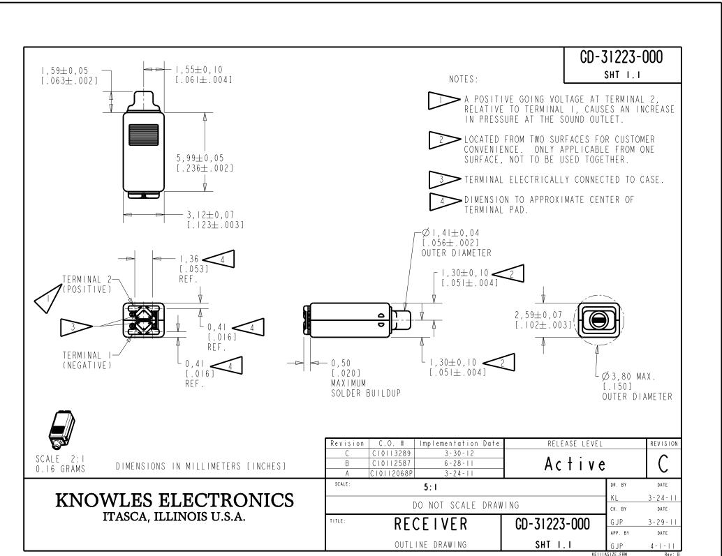
INTENDED FOR USE IN CIC, RIC, AND MINI-BTE APPLICATIONS. THIS IS A PAIR OF GE RECEIVERS WITH VERY LOW VIBRATION IN ALL DIRECTIONS. ONE GE RECEIVER IS REVERSE MAGNETIZED FOR MAGNETIC LEAKAGE CONSIDERATIONS. BOTH DAUGHTER UNITS HAVE THE CENTER TERMINAL CONNECTED TO CASE.
