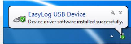
8 You have successfully installed the necessary software and driver for your EL-USB-ACT data logger. An 'EasyLog USB' icon will be placed on your desktop.
