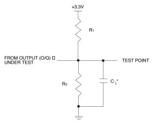
$^{\star}\text{C}_{\,\text{L}}$  INCLUDES TEST FIXTURE AND PROBE CAPACITANCE
