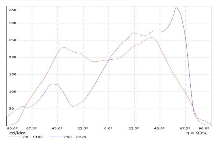
Luminaire: LEDiL Oy STRADA-SQ-T4\_(MK-R) Lamps: 1 x CREE\_MK-R\_356.736lm@250mA\_P=2.83786W\_I=249.9mA
