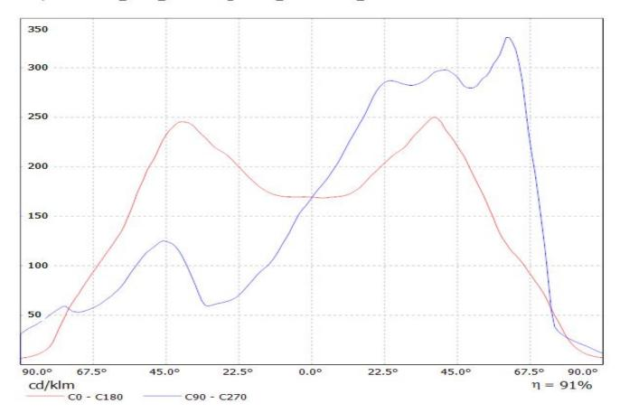
Luminaire: LEDiL Oy STRADA-SQ-T4\_(LuxM) Lamps: 1 x Luxeon M LXR7-SW30 360Im@250mA CCT:3000K
