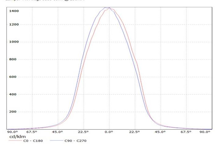
Luminaire: Ledil Oy CA12350\_TINA2-W (Avego Jade 69Im @ 250mA) Efficiency=90% Lamps: 1 x Avego Jade 69Im @ 250mA
