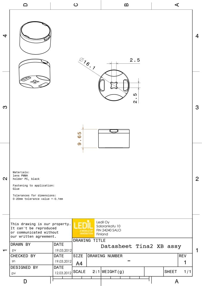
Luminaire: Ledil Oy CP12674\_TINA2-W (Cree XB-D 94Im @ 250mA) Efficiency=81% Lamps: 1 x Cree XB-D 94Im @ 250mA
