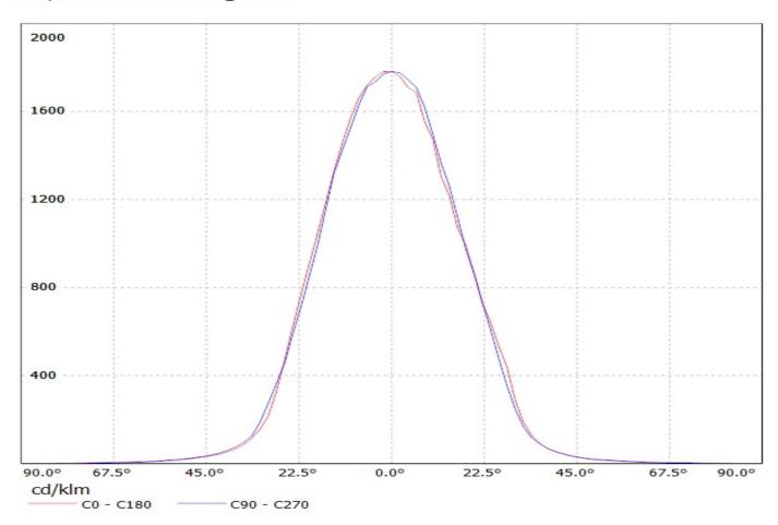
Luminaire: Ledil Oy CP12674\_TINA2-W (Cree XB-D 94lm @ 250mA) Efficiency=81% Lamps: 1 x Cree XB-D 94lm @ 250mA
