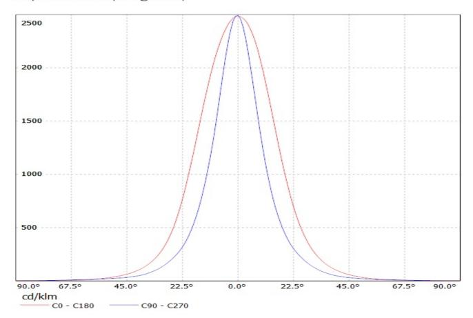
Luminaire: LEDIL OY CP12684\_TINA2-O / CA11173\_TINA2-O (Cree MX-6) Efficiency=85% Lamps: 1 x Cree MX-6 (67Im @ 250mA)
