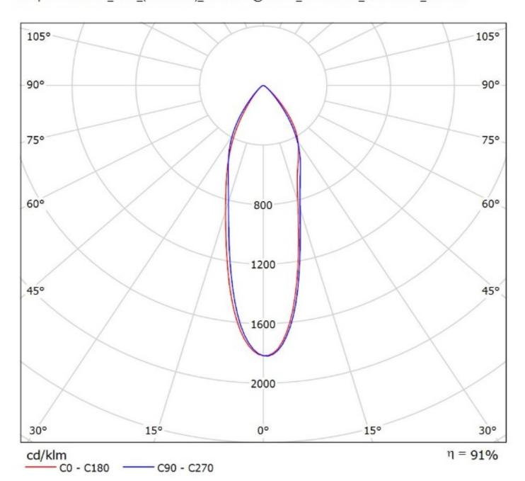
Luminaire: LEDIL OY FA11019\_Tina-WW (Cree XP-G) Efficiency=91% Lamps: 1 x Cree XP-G (92Im@250mA)
