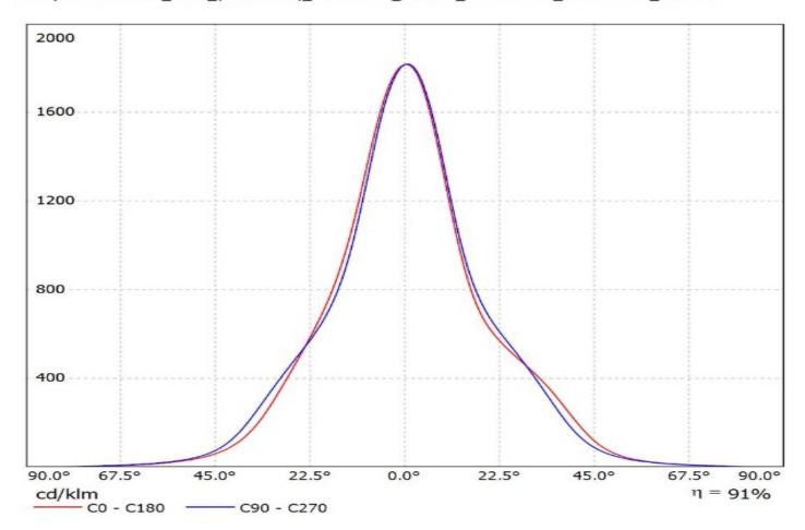
Luminaire: LEDIL OY FA11019\_Tina-WW (Cree XP-G) Efficiency=91% Lamps: 1 x Cree XP-G (92Im@250mA)
