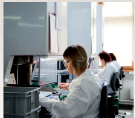
Ultrasonic welding of sockets
