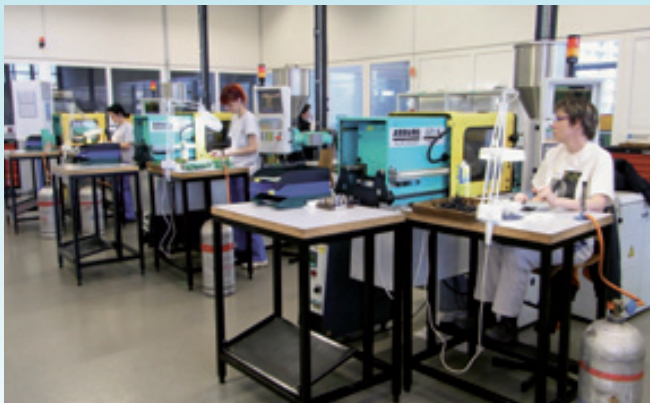
Plastic moulding of bend reliefs
