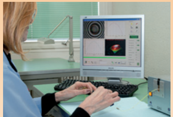
Inspection of fibre optic polishing
