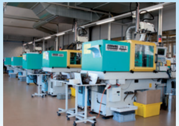
Injection of insulators
