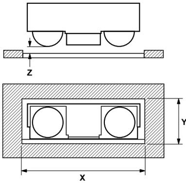
X is the width of the window, Y is the height of the window, and Z is the distance from the HSDL-3201 to the back of the window. The distance from the center of the LED lens to the center of the photodiode lens is 5.1 mm. The equations for the size of the window are as follows:
