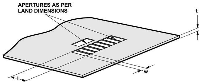
Aperture opening for shield pad is 2.7 mm x 1.25 mm as per land pattern.
