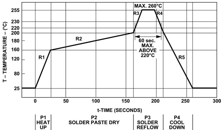
The reflow profile is a straight-line representation of a nominal temperature profile for a convective reflow solder process. The temperature profile is divided into four process zones, each with different  $\Delta T/\Delta \text{time}$  temperature change rates. The  $\Delta T/\Delta \text{time}$  rates are detailed in the above table. The temperatures are measured at the component to printed circuit board connections.
