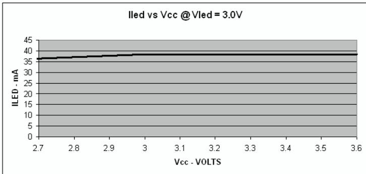
**Figure 1. LED current vs. Vcc.**
