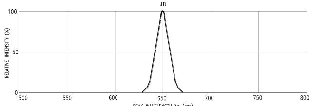
PEAK WAVELENGTH  $\lambda p$  (nm) Fig1.Spectral Emission
