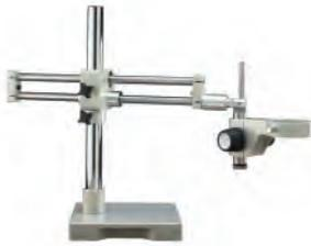
**23730RB**, this Dual Boom Ball-Bearing Stand features a 26" stainless steel horizontal boom extension (limited to 24" when used with a System 373 model) and a 17½" vertical boom mounted to a 10" x 10" die-cast base. Ball-bearing design allows fluid horizontal extension of the boomstand. The focus mount angles to 45° to permit additional viewing and inspection perspectives.
