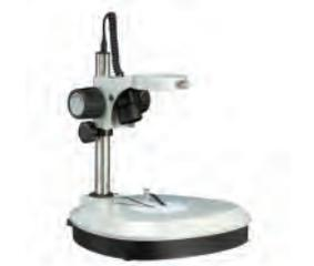
**23733**, an illuminated stand used for viewing small objects. Two independently controlled light sources. A dimmable 10-watt halogen light is focused on the subject and a 5-watt compact fluorescent lamp provides back lighting from underneath through a translucent medium. Base of stand is 11½" wide by 11½" deep, the vertical post is 11" high (measured from surface to top of vertical post).
