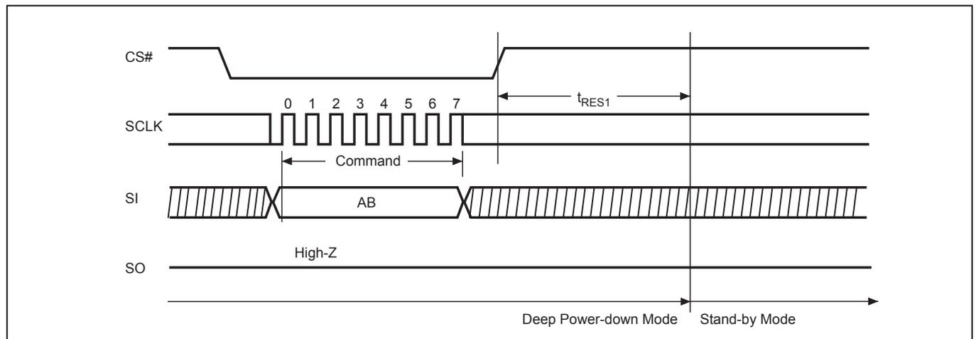
**Figure 24. Read Electronic Signature (RES) Sequence (Command AB)**
