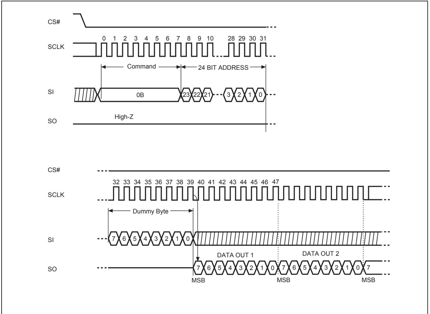
**Figure 17. Dual Output Read Mode Sequence (Command 3B)**
