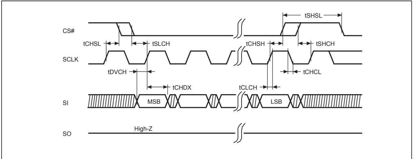
**Figure 8. Output Timing**
