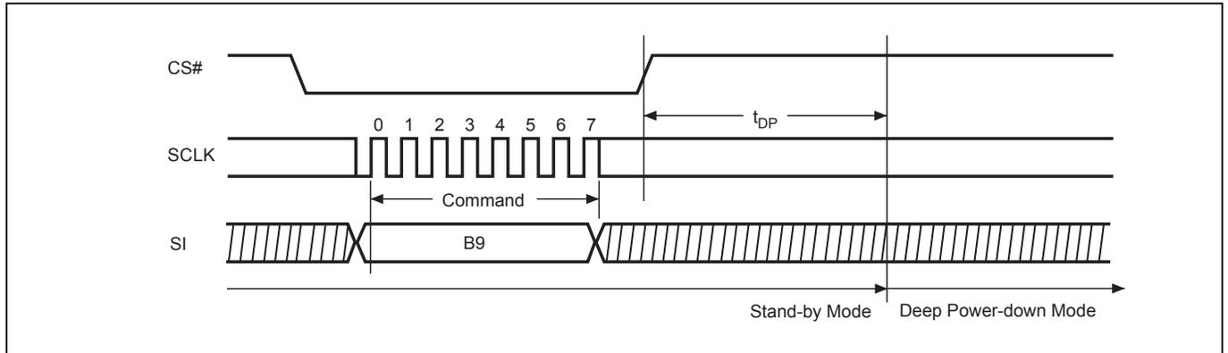
**Figure 23. Release from Deep Power-down (RDP) Sequence (Command AB)**
