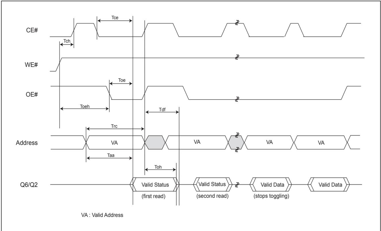
Figure 16. TOGGLE BIT ALGORITHM
