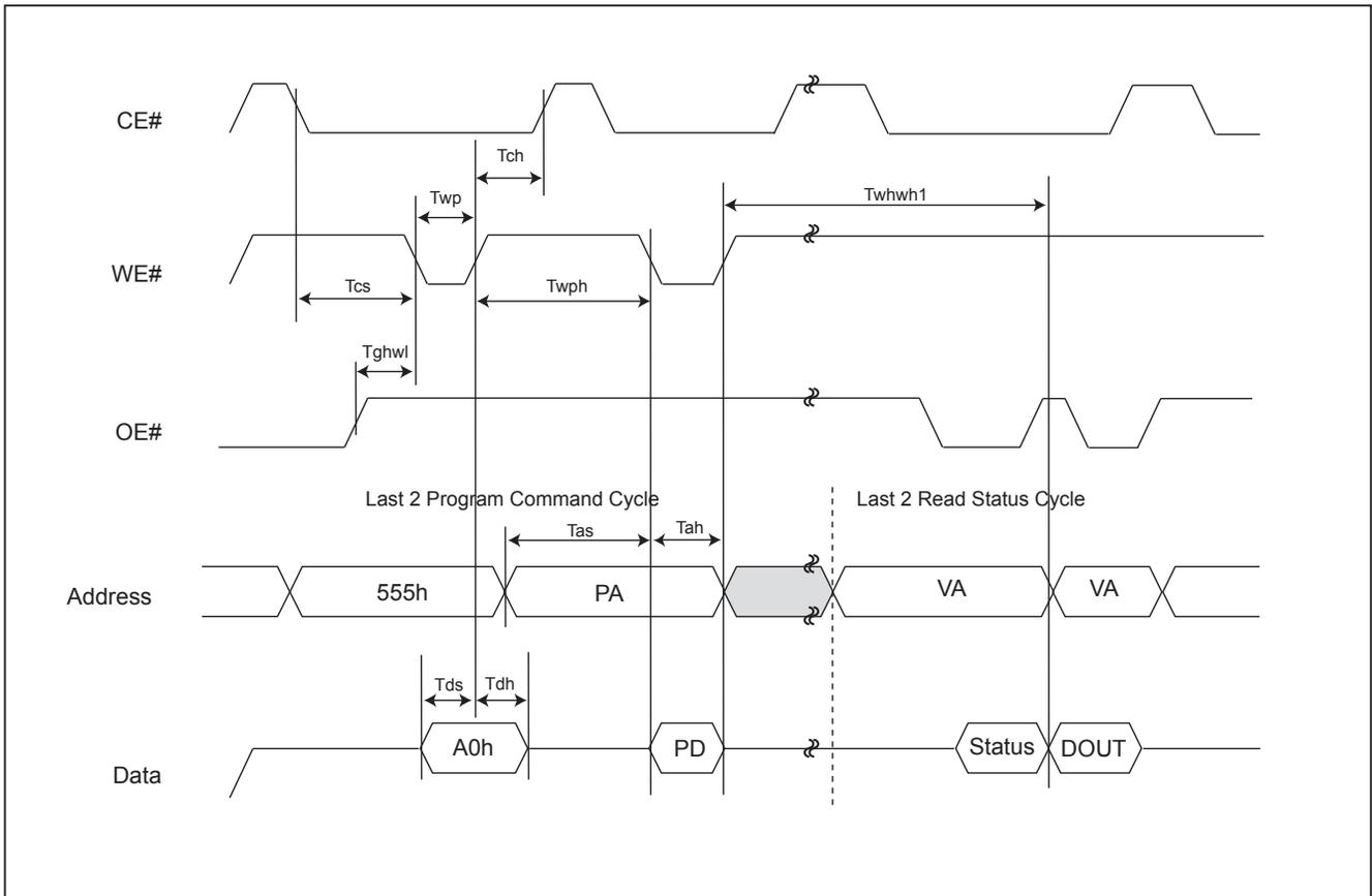
**Figure 9. CE# CONTROLLED WRITE TIMING WAVEFORM**
