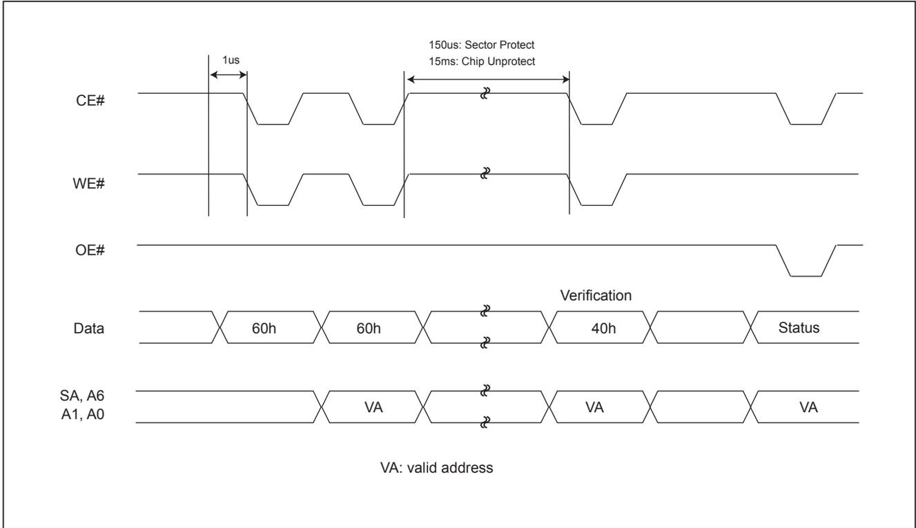
**Figure 12. SILICON ID READ TIMING WAVEFORM**
