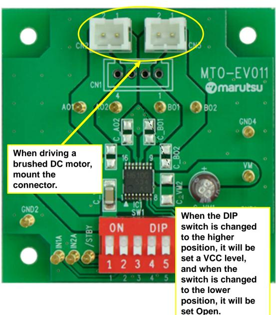
This evaluation board has a DIP switch (SW) so that the operation setting of the TC78H621FNG can be set without the external signal input.
