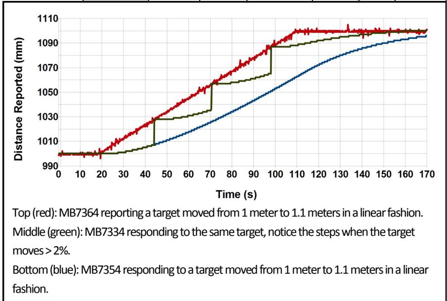
The MB7334 and MB7344 have an additional filter similar to the MB7354 and MB7374 except that the filter will reset to targets that are considered valid outside of a 2% distance to target window. This makes the sensor an ideal balance for accurately monitoring slow or stationary targets that occasionally move rapidly.
