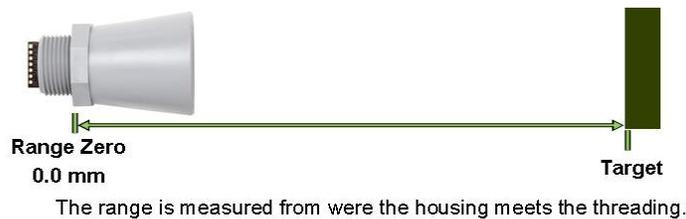
In general, the HRXL-MaxSonar-WR will report the range to the leading edge of the closest detectable object. Target detection has been characterized in the sensor beam patterns.
