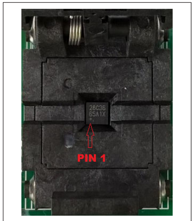
Figure 9. Orientation of the DS28C36, DS28E36, and DS2476 in the Burn-In Socket
