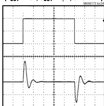
LOAD TRANSIENT ( V_{OUT} = 10V , C_{OUT} = 1\mu F , 0 TO -2mA)
