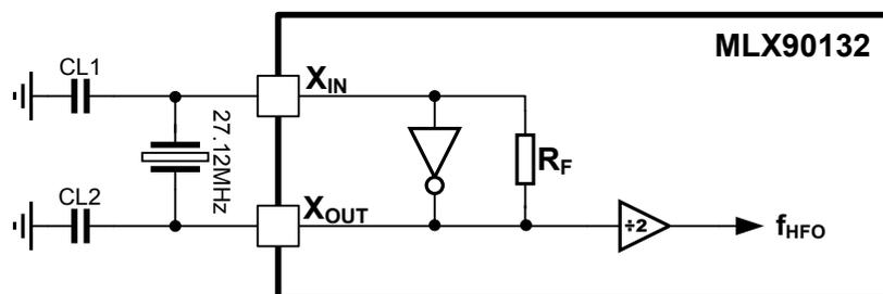
**Figure 15: Typical application with a 27.12MHz crystal**
