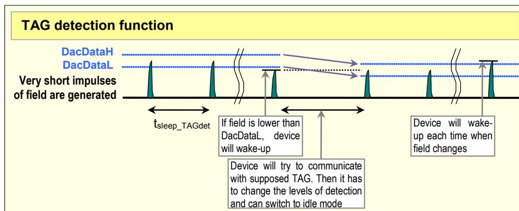
**Figure 10: MLX90132 TAG detection principle**
