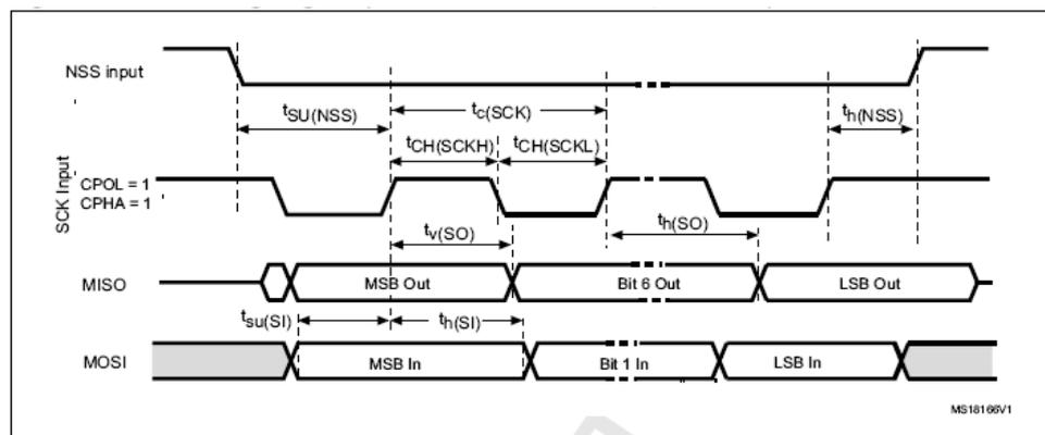
**Figure 14: SPI timing diagram (Slave mode and CPOL = 1, CPHA = 1)**
