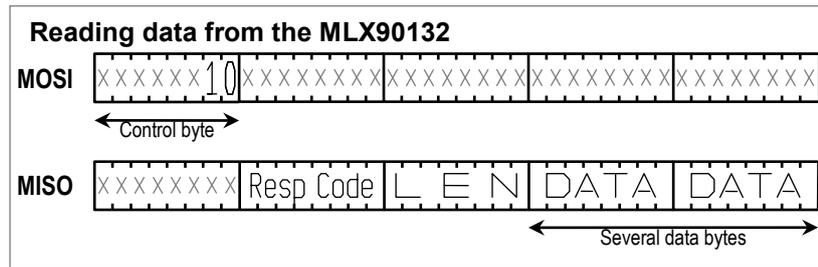
**Figure 8: SPI communication, reading data from the MLX90132**
