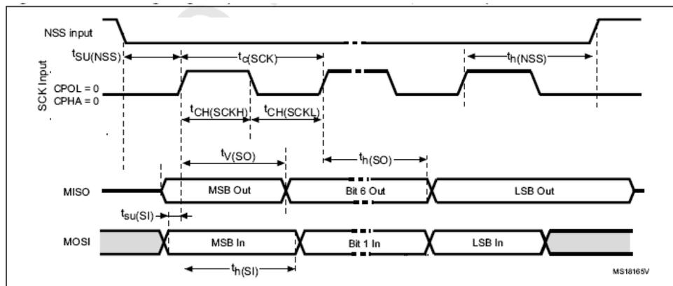
**Figure 13: SPI timing diagram (Slave mode and CPOL = 0, CPHA = 0)**
