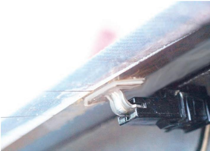
Very effective at bonding car rear defrost tabs back on the grid permanently.
