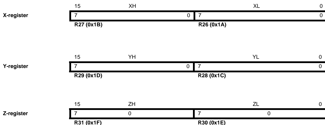
Figure 4-3. The X-, Y-, and Z-registers
