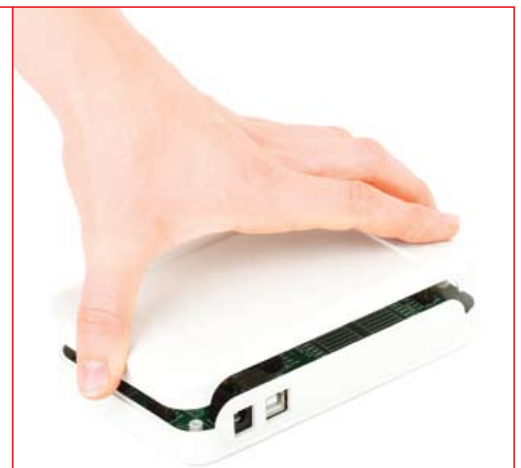
Figure 8-3: Place plastic casing cover and wind screws into outer screw holes to fix it with bottom plastics casing
