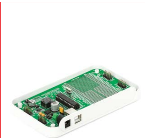
Figure 8-2: Wind screws into inner screw holes to fix the board with the bottom plastic casing
