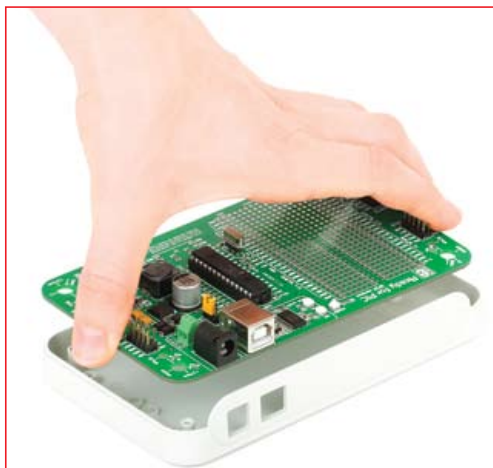
Figure 8-1: Place the board into the bottom part of the casing. Make sure that connectors are aligned with square openings
