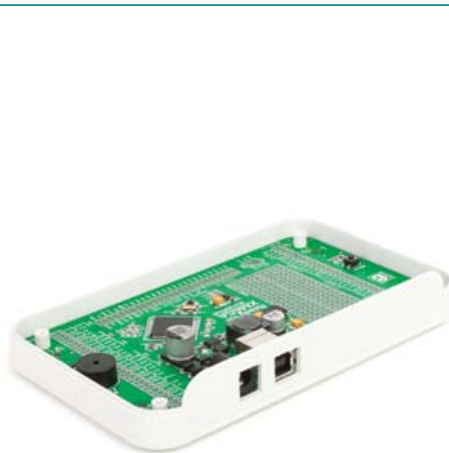
Figure 9-2: Wind screws into inner screw holes to mount the board to the bottom casing plastic
