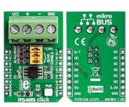
RS485 Click 5V is an accessory board in mikroBus<sup>TM</sup> form factor. The on-board ADM485 differential line transceiver is suitable for high speed bidirectional data communication on multipoint bus transmission lines. It is designed for balanced data transmission and complies with EIA standards RS-485 and RS-422. This transceiver features a differential line driver and differential line receiver. Board is set to use 5V power supply only.
