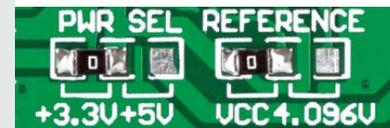
There are two zero-ohm resistors (SMD jumpers): **PWR SEL** is used to determine whether 5V or 3.3V power supply is used, and **REFERENCE** to select either VCC or 4.096V as the voltage reference.
