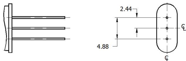
**Note:** This drawing is intended for lead dimension only. Please refer to the appropriate MMD Spec Sheet for addition package dimensions.
