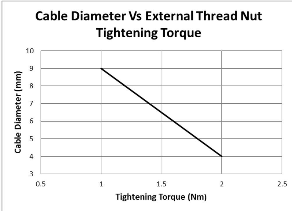
Graph showing external thread tightening torque for Form A & B.
