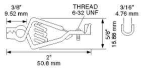
BU-48B Steel Automotive Analyzer/Test Systems Clip - 10 Amp or, BU-48C Solid Copper - 20 Amp
