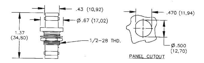
BNC Body is isolated from the mounting flange Mounts in panels up to .175" (4.45) thick
