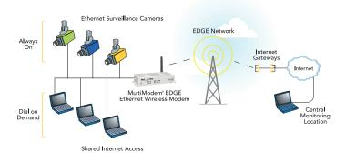
**Industry-standard Modem Commands.** The MultiModem EDGE wireless modem provides industry-standard AT-style commands for ease of integration into your existing software application.
