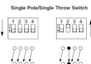
NB: The D1U54x Series employs "left shifted" 7-Bit addressing; where Bit "0" of the device address is the Read/Write bit. The addresses, as shown above, assume that the Read/Write bit is a logic level "0".
